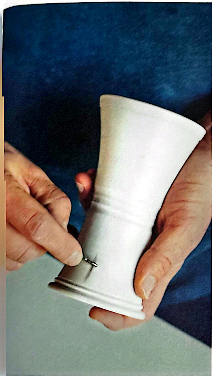
The scratch test is a quick way to tell whether silverware is likely to leave a similar mark on functional work.
