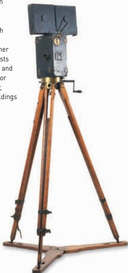
» **This silent movie camera** stands on top of a sturdy tripod, and was cranked by hand.
