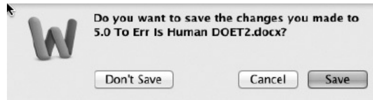
FIGURE 4.6 A Lock-In Forcing Function. This lock-in makes it difficult to exit a program without either saving the work or consciously saying not to. Notice that it is politely configured so that the desired operation can be taken right from the message.
