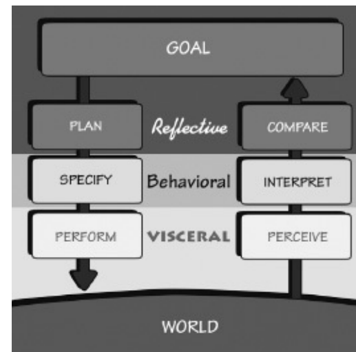
FIGURE 2.4. Levels of Processing and the Stages of the Action Cycle. Visceral response is at the lowest level: the control of simple muscles and sensing the state of the world and body. The behavioral level is about expectations, so it is sensitive to the expectations of the action sequence and then the interpretations of the feedback. The reflective level is a part of the goal- and plan-setting activity as well as affected by the comparison of expectations with what has actually happened.
