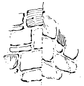
Fig. 188. This is wrong: stones do not match at the outer corner of the building.
